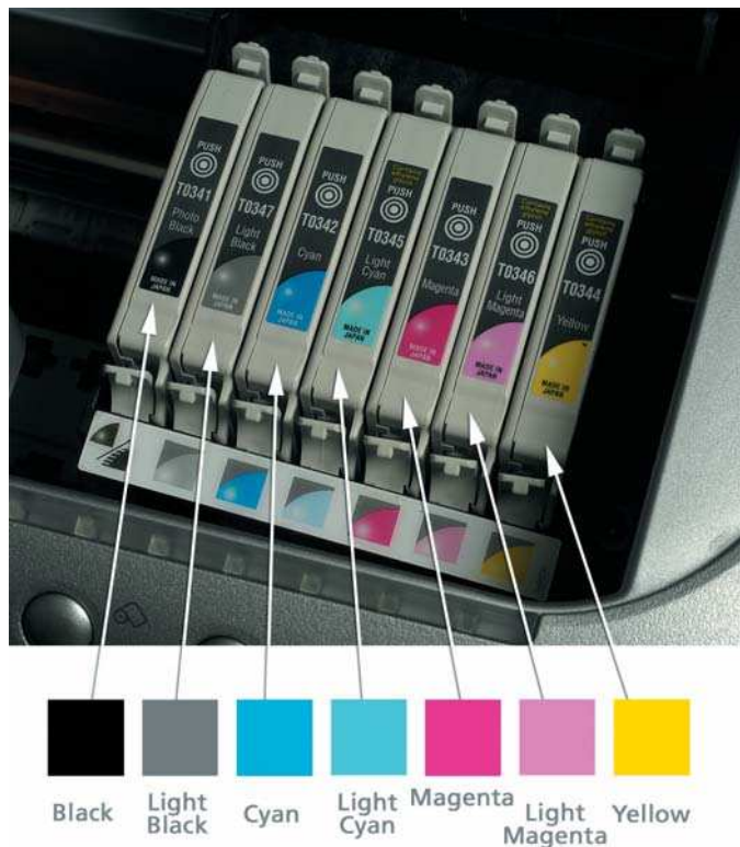
Figure 31.2 Inkjet printers designed especially for photographic printing often contain five colors plus black, and some models can even print up to A3+ (bigger than A3).
